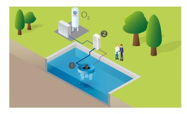
One version of the **OXY INJECTOR-TURBOXAL** system is able to suck air or off-gas from an ozone reactor at low pressure.
